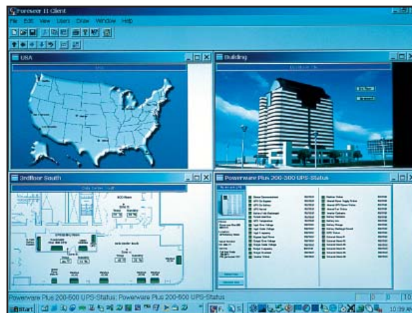
A configurable user interface displays critical data center information with FORESEER software.
